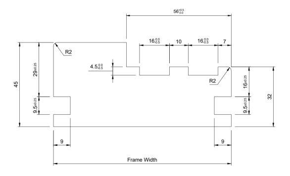
Do Not Scale. Description: Purchasing Profile Timber System 2 - 44\_32 Profile - FD60 - 54mm Door - Non-Acoustic - Q2F To Both
